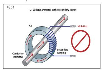
In fig b, when secondary circuit is open, there is no secondary current 12 and hence counterbalancing flux  $\emptyset$  2 is absent and hence Net flux  $= \emptyset = \emptyset$  1 which is very large and this produces a very high back emf as per Lenz's equation.
