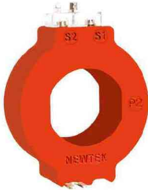
Mounting Arrangement CT ID 65X20 CT OD 118(L)X100(W)X40(T) Primary Bar 60X10mm
